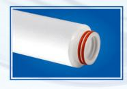
Polypro-226: Also known as sanitary cartridge filters, Type 226's have double gaskets which are similar to the Type 222. Locking fins are included with this type of cartridge, which ensures proper installation of the filter. When installing this type of cartridge into the sanitary cartridge filter housing, it must be properly lined up with the opening and twisted as it is pushed in. This ensures a full lock and proper bypass protection.
